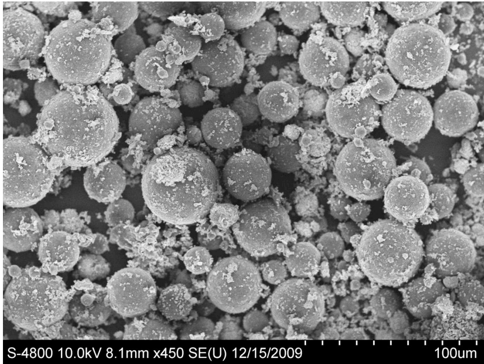
Figure 2.5 (a) Palacos R polymer beads with visible zirconium dioxide molecules and (b) Surface of one Palacos R polymer bead showing dispersion of MWNTs and zirconium dioxide.
